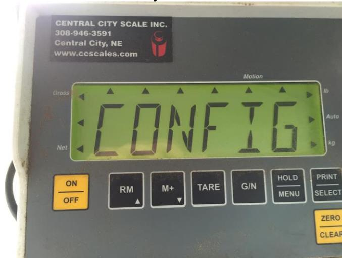
6. Now use the menu button to move to the right and the select button to select the path or option to navigate the chart below. So for the first step hit the menu button until the display says “RS232” and then press select. The display should now say “PORT 1”.
